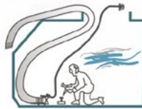
Welding gas removal
