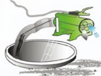
Supply of fresh air and removal of harmful gases
