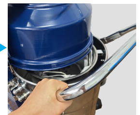
After separating collection tank, remove the sludge
