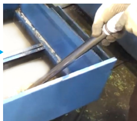
Discharge of filtered cutting fluid and oxygen supply
